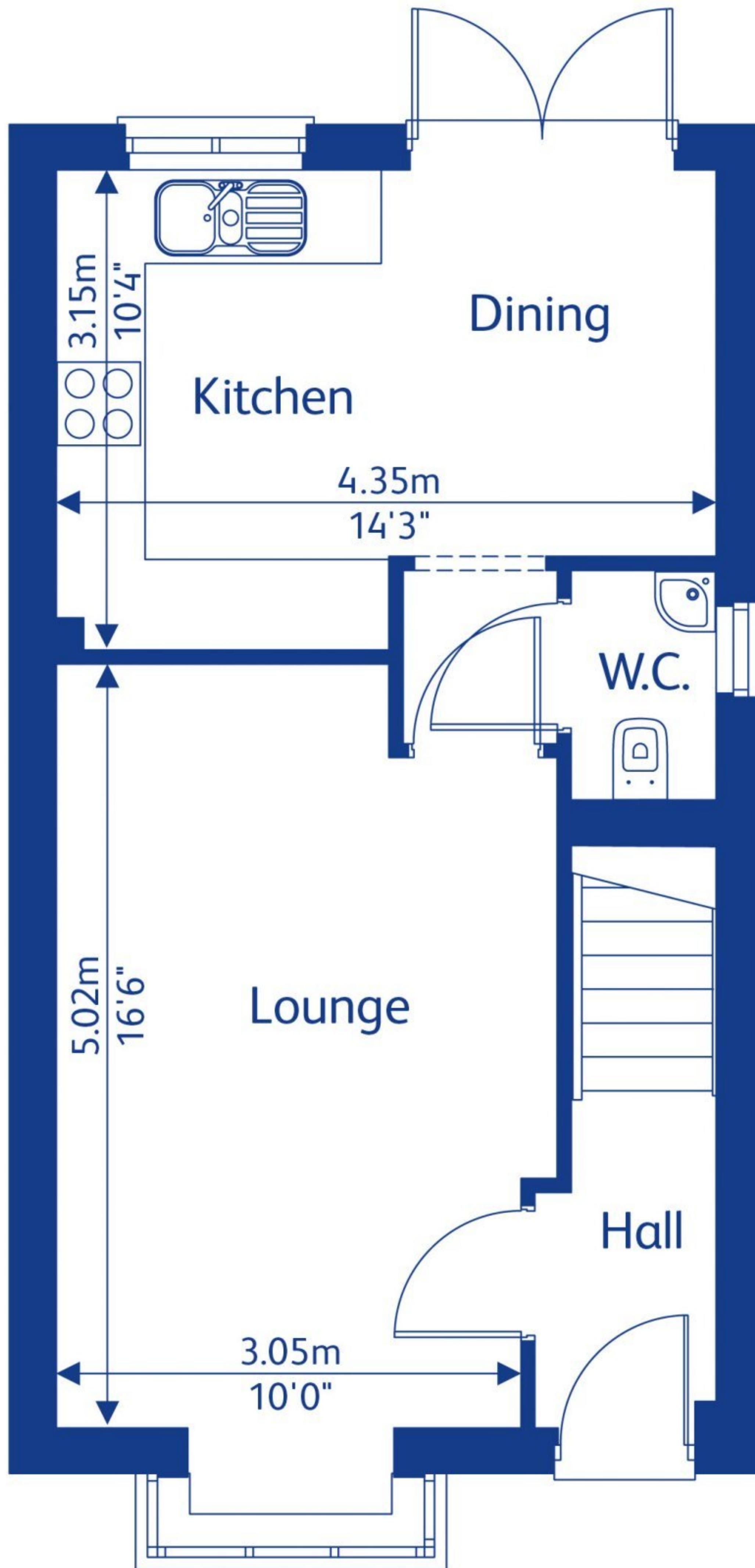
Note: All dimensions are maximum and account for alcoves, and a tolerance of  $\pm 75\text{mm}$  should be allowed.
